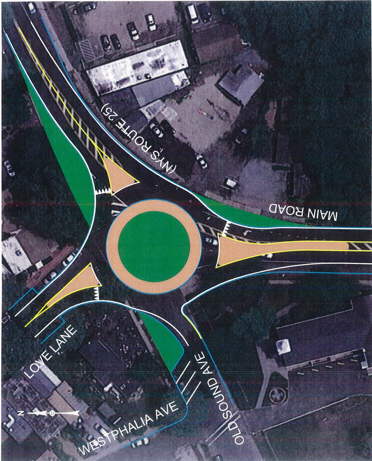
FIGURE 11 CONCEPTUAL DESIGN PLAN FOR POSSIBLE ROUNDABOUT MAIN ROAD (ROUTE 25) AT LOVE LANE/ OLD SOUND AVENUE
